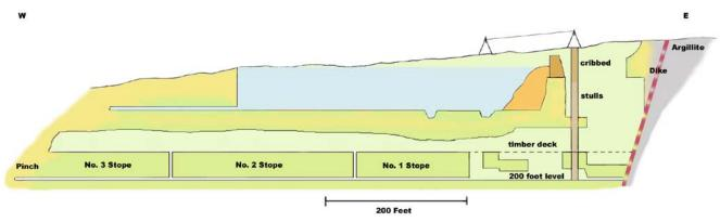
Figure 13: Showing the stopes worked between 1938 and 1939.
