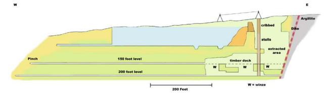
Figure 10: Showing the location of the three winzes and rail track timber deck.
