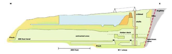
Figure 15: Showing the second winzes and pinch on the lowest level in 1940.
