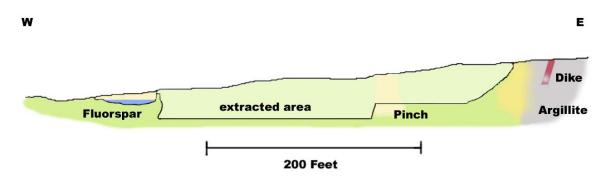
Figure 3: The open-cut by the end of November 1933.
