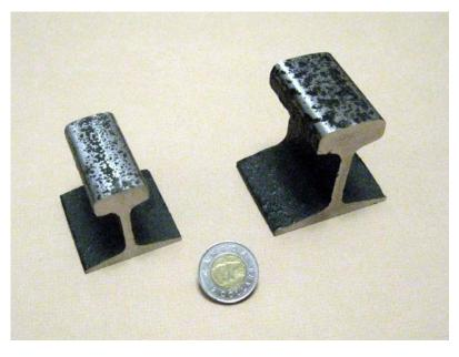
Figure 18: 12lb and 20lb Rail Sections from the Black Duck Mine.
