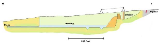
Figure 7: Showing flooding and the placement of the dam, backfill and east shaft.
